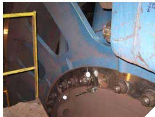
Adjustments to the gear – axial and radial
