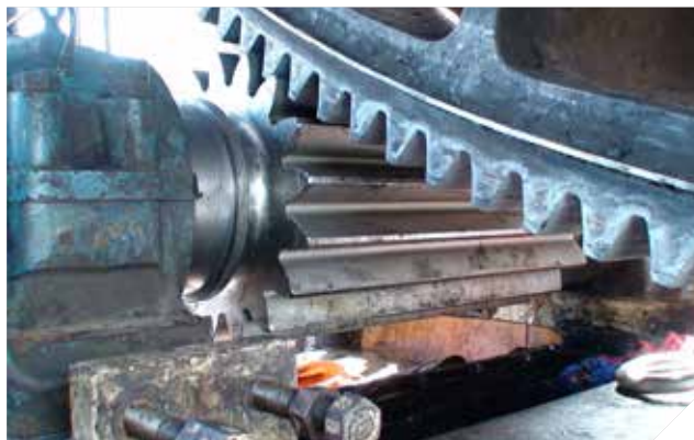
Pinion being aligned to the reversed gear
