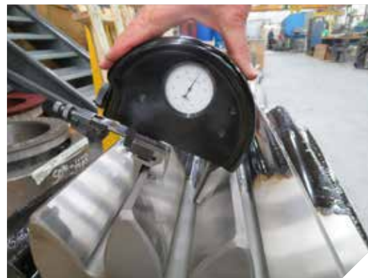
Measuring critical parameters of the pinion
