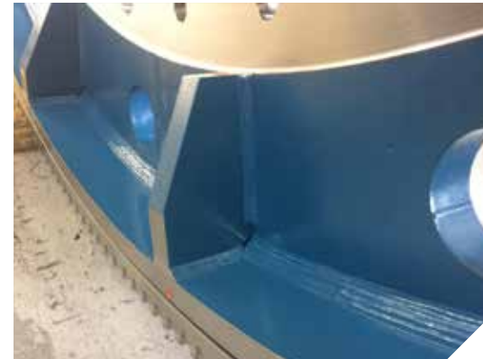
Replacing a previously cast gear with a new welded design
