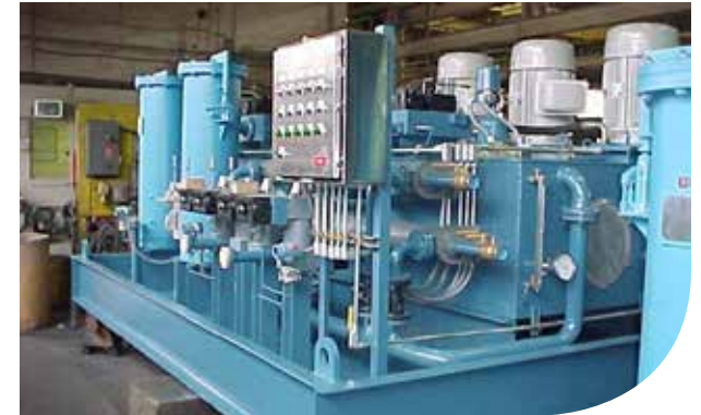
Hydrostatic lubrication system
