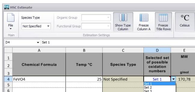
**Fig. 3.** Changing the active set of oxidation numbers.
