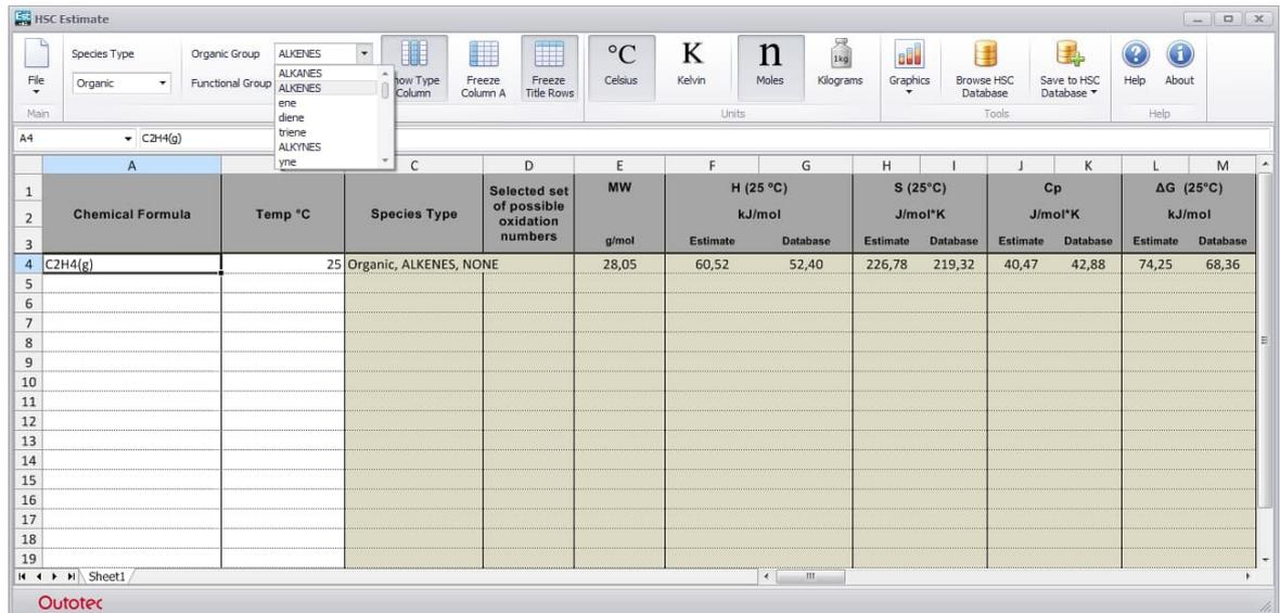
**Fig. 2.** Specifying additional properties for organic species (C<sub>2</sub>H<sub>4</sub>(g) in this example).
