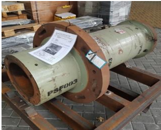
Pinion shaft Primary crusher
