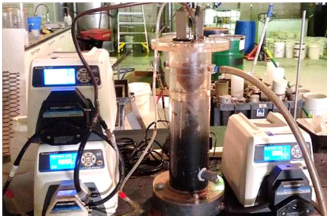
99mm Diameter Lab Scale Thickener used for laboratory dynamic thickener testwork.
